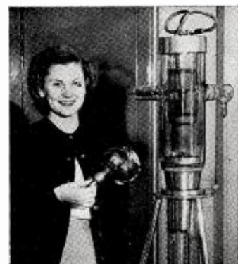
WWVA receptionist Gladys Stempien holds original tube (50 w power) used when station first went on air in 1926. To her left is one of 100,000 w tubes used in the new WWVA 50 kw transmitter.
