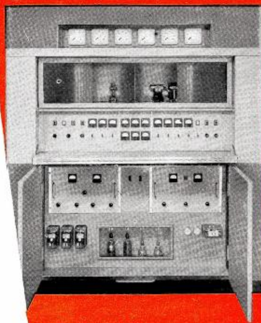
Smartly styled FM transmitters (in two-tone blue and grey) are built in lightweight aluminum cabinets to facilitate portability and rapid installation.
